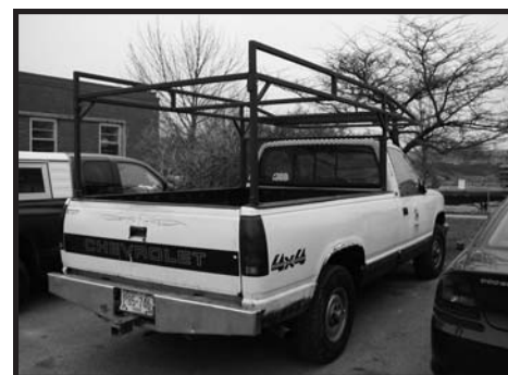
Pickup truck with the ladder transport rack fabricated for Habitat for Humanity.
